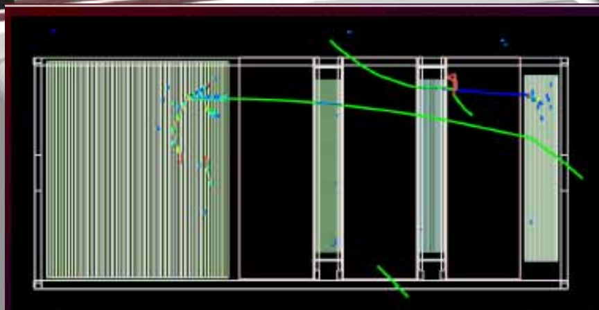
A CC1 \pi interaction in the P0D, with full-bunch background
