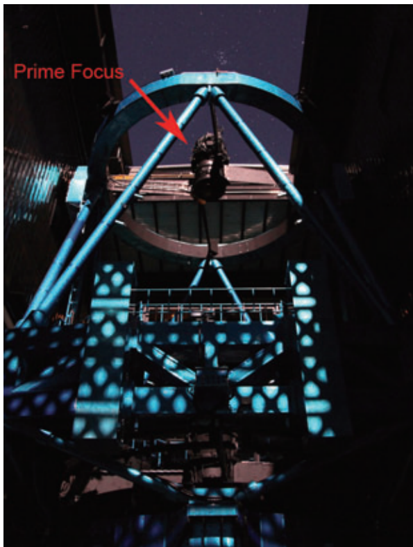
The 8.2m Subaru Telescope and the HSC camera. The image on the left shows the position of HSC (without the filter exchange unit or FEU) when mounted on the inner, top ring of the Subaru Telescope. This location is at prime focus, and HSC is 15 meters above the primary mirror. (Credit: NAOJ). The image on the right is the 3m tall HSC camera. (Credit: NAOJ)
