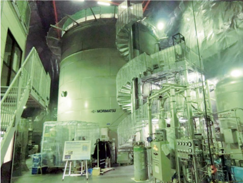
The XMASS hall with its water shield tank
