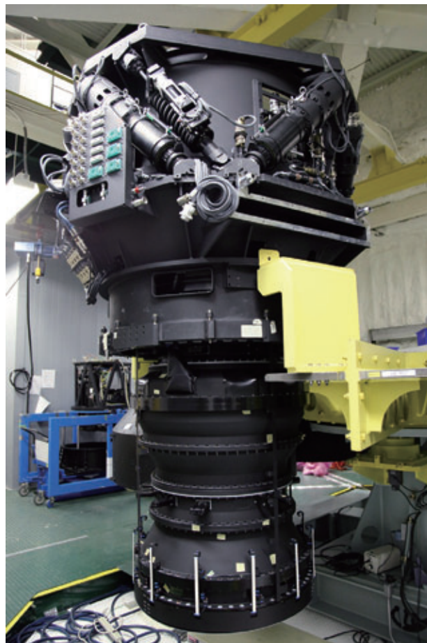
The 8.2m Subaru Telescope and the HSC camera. The image on the left shows the position of HSC (without the filter exchange unit or FEU) when mounted on the inner, top ring of the Subaru Telescope. This location is at prime focus, and HSC is 15 meters above the primary mirror. (Credit: NAOJ). The image on the right is the 3m tall HSC camera. (Credit: NAOJ)
