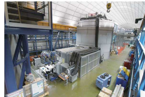
Figure 1: XENONnT’s 700-ton water shield tank from the back of Hall B at the Gran Sasso Underground Laboratory (LNGS). On the left part of the Gd-water system sticks out from behind the gray cleanroom guarding the installation port of that water tank. Photo by Kai Martens.
