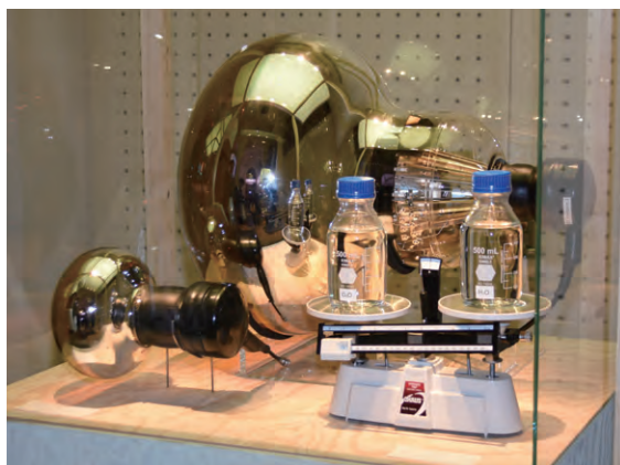
Photo 1: A 20-inch PMT and an 8-inch PMT for the Super-Kamiokande experiment and heavy water ( D_2O ) used in the SNO experiment and light water ( H_2O ). They were donated to the Nobel Museum.
