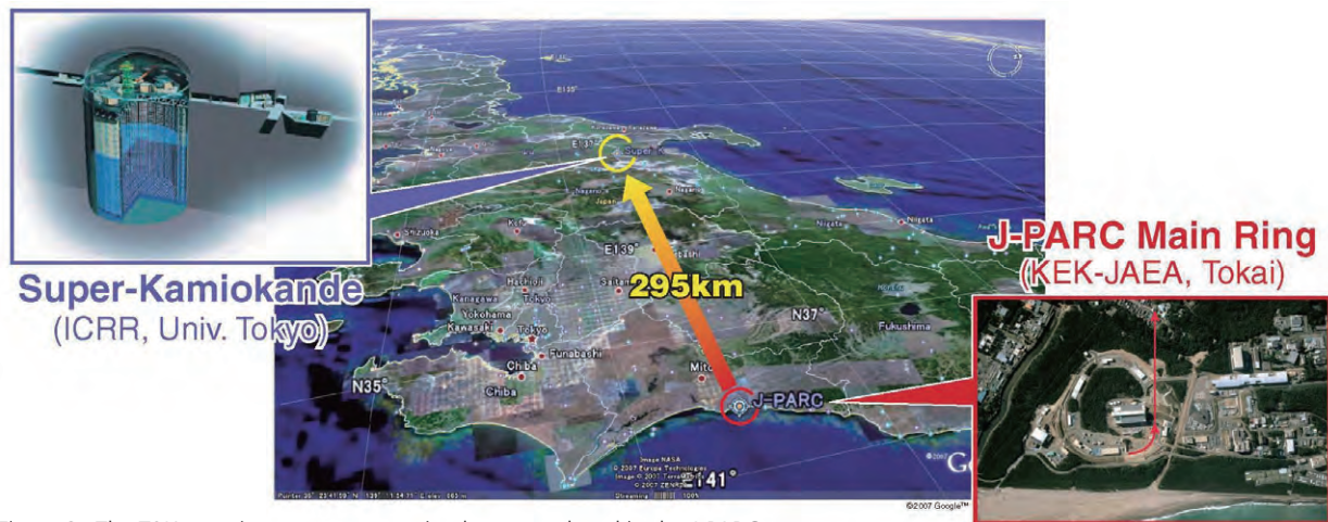
Figure 3. The T2K experiment uses a neutrino beam produced in the J-PARC facility in Tokai-mura on the east coast of Japan. A small fraction of the neutrinos are detected at the Super-Kamiokande detector located 295 km away.
