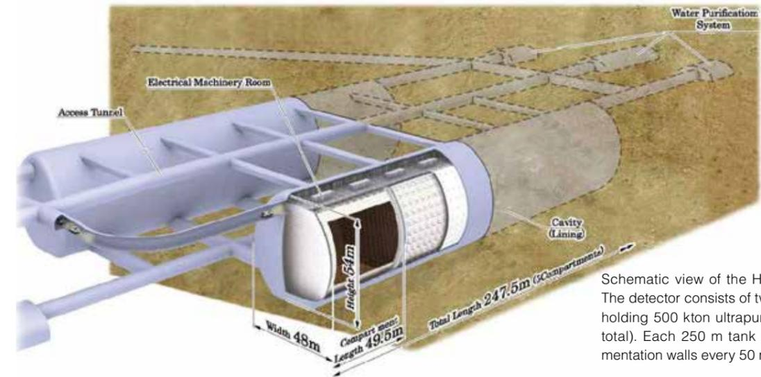
Schematic view of the Hyper-Kamiokande. The detector consists of two cylindrical tanks holding 500 kton ultrapure water (1 Mton in total). Each 250 m tank is divided by segmentation walls every 50 m.
