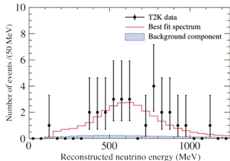
Fig. 1: The reconstructed energy of the observed  $\nu_e$  candidate events, and the prediction with no  $\nu_\mu \rightarrow \nu_e$  oscillations (blue) and with  $\nu_\mu \rightarrow \nu_e$  oscillations (red).
