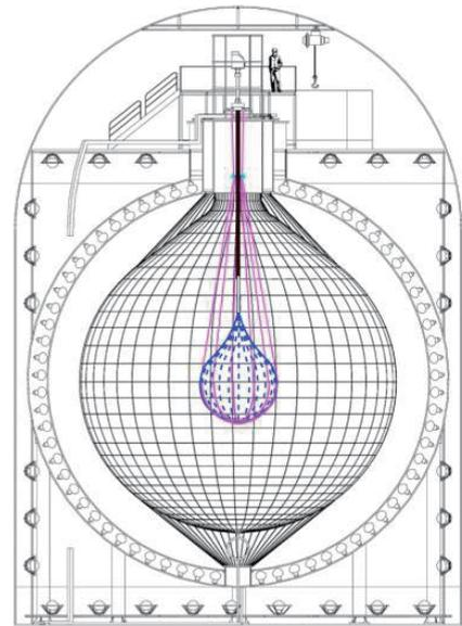
Figure 3: A schematic of the KamLAND-Zen detector.
