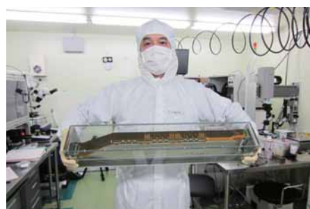
Figure 2: Photograph of a dummy ladder for the outermost SVD layer with a slant structure in the forward region (right side of the snapshot). Photograph was taken in our clean room.
