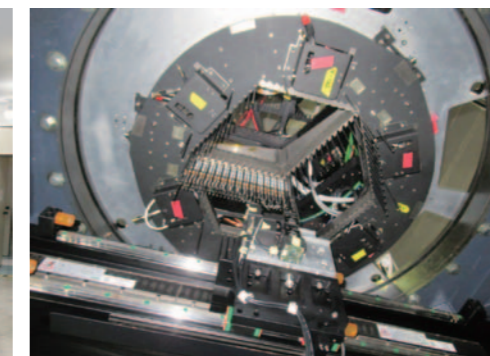
Figure 3: Left -- The fiber cable under integration at Laboratório Nacional de Astrofísica (LNA) in Brazil that will be installed on the telescope and will transmit light from the Prime Focus Instrument on the Subaru prime focus to Spectrograph System. Right -- The focal plane of Prime Focus Instrument under integration by ASIAA and their partner ASRD (Aeronautical Systems Research Division) of CSIST (Chung-Shan Institute of Science and Technology) in Taiwan.
