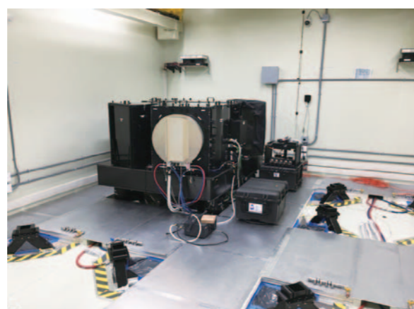
Figure 2: The first spectrograph module fully reassembled in the dedicated clean room in the Subaru telescope enclosure building.
