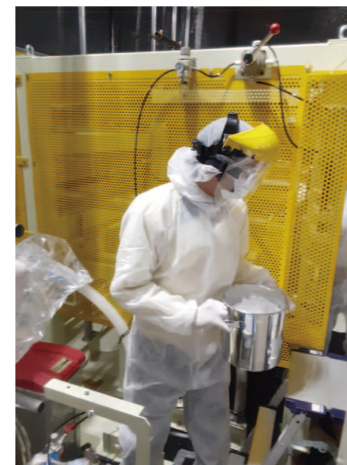
Figure 2: Carrying pure gadolinium sulfate to be dissolved and injected into Super-K.
